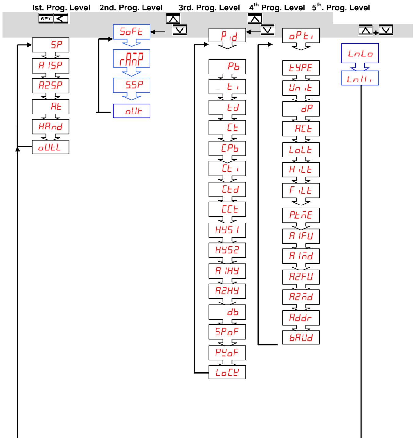
1. When 2<sup>nd</sup> Output (Cooling) is not selected, CPb·Cti·Ctd·HYS2 and db parameters are not available.
