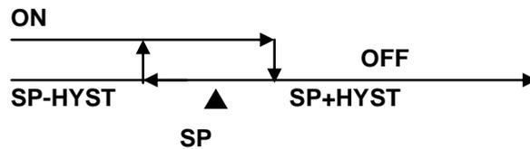
When the second control output (output 2 cooling) is fitted it will behave as shown below. Bear in mind that when using Proportional or PID control there may be an overlap between the heating and cooling depending on the auto PID algorithm calculations. This is perfectly normal. You can make both heating and cooling proportional band = 0 then it will ensure that between the two nothing is switched on.
